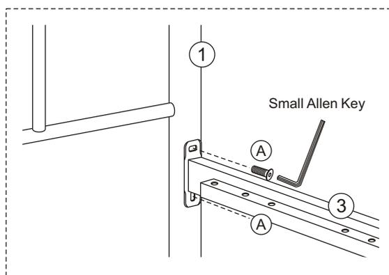
**IMPORTANT:** Do not tightly secure the screws before completing Step 2.
