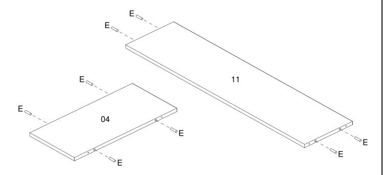
**Step 3:** Insert hardware part E using small mallet (not provided). **DO NOT use any power tools as this may damage the frame and will invalidate any claim.**
