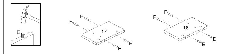
Step 2: Insert hardware part E using small mallet (not provided).
