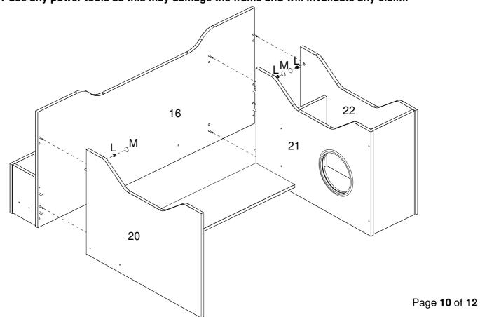
**Step 16:** Attach hardware part A2 to the o the lower left side (20), lower division (21) and lower right side (22) using hardware part N and small mallet (not provided).
