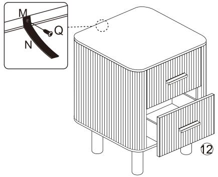
PLEASE NOTE that wall fixings are not supplied as different wall materials require different fixing devices. You must use fixings devices suitable for the type of wall you intend to mount product to. Ensure the head of any screw used has a diameter greater than the mounting hole and the fixing is safe and secure before use.
