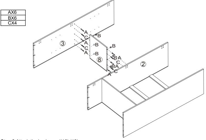
Step 6:Attach the back panel(16),(18).
